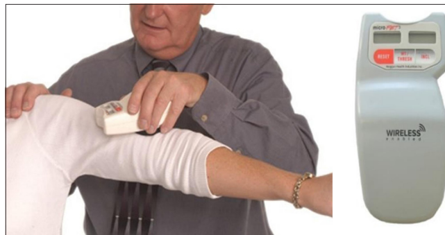
Figure 3: Hand-held digital inclinometer-by Hoggan Health used to measure the range of motion of shoulder forward flexion (range of motion of shoulder forward flexion)
